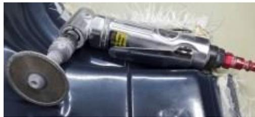
Diamond blade cut off tool w/ 20k rpm side angle cutoff tool cost at (Harbor freight \$14.95).
